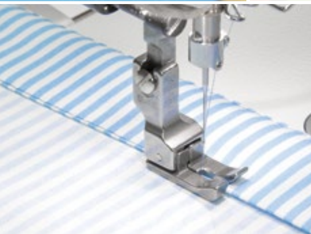
TEXI 5015 Foot with central tape guide 4.8 mm
